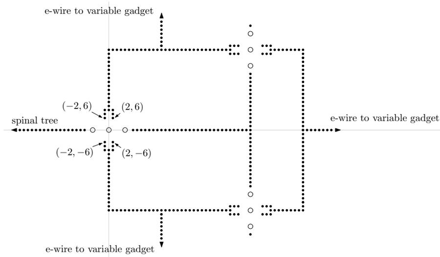
**Fig. 8** The configuration used for the clause gadgets, with the gadget placed in the canonical position. The filled small circles (black dots) are disks of radius 0, while the larger empty circles are unit disks. A wire extends from the gadget as part of the spinal tree, and three e-wires go to three variable gadgets (one for each literal in the corresponding clause of the 3-SAT instance).
