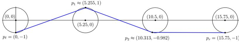
**Fig. 10** The optimal setting for Case 1. The optimal point in the first separating disk is slightly to the right of the extreme upper point in the disk, while that of the second disk is nearly  $11^\circ$  clockwise of the extreme lower point. Despite these differences, the change in path weight between this optimal path and a path using the extreme points is less than 0.01 units.
