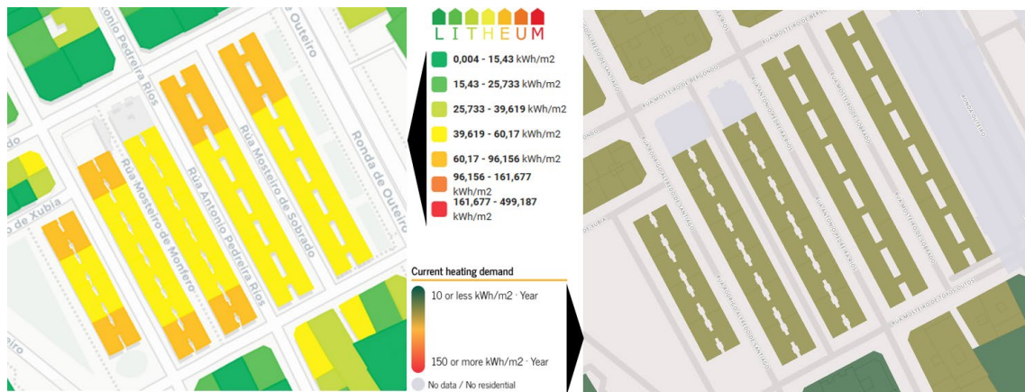
Fig. 19 The energy model in Litheum takes into account the obstruction angle and envelope exposure of each building, (left). The map on the right shows the same area as represented by the Urban3R project (Ciclica, 2023)
