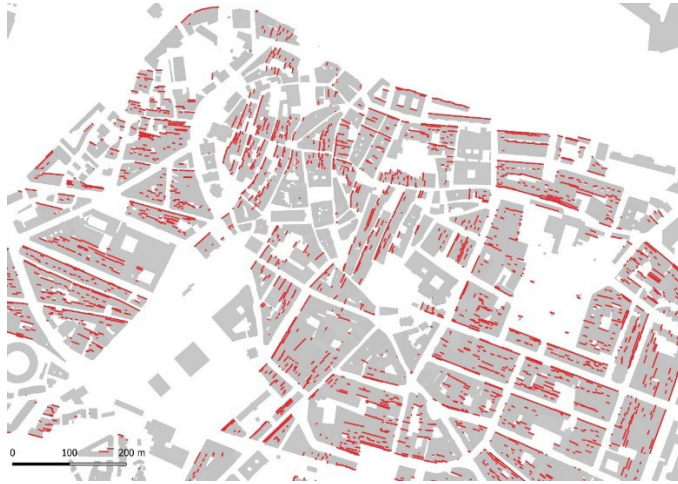
Fig. 9 Exposed segments by orientation quadrants as part of the calculation process of the exposed envelope
